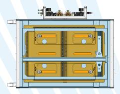
The device Is equipped with 4 nozzle adjustable in 4 direction to fit with every box, and a gel bar with 14 needle that moves trough the cabin to cover all the chick box.
